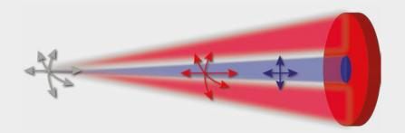
Working principle of the delay unit. The time delay is introduced by changing the core position (reflecting the XUV/soft X-ray pulses) with respect to the ring (reflecting the IR pulses). The 5 degrees of freedom offer perfect control for spatial and temporal overlap in the focus.
