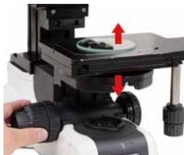
Adjustable stage height for varying sample sizes
