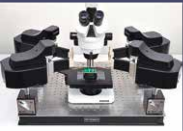
Installation example for 4-terminal measurements
