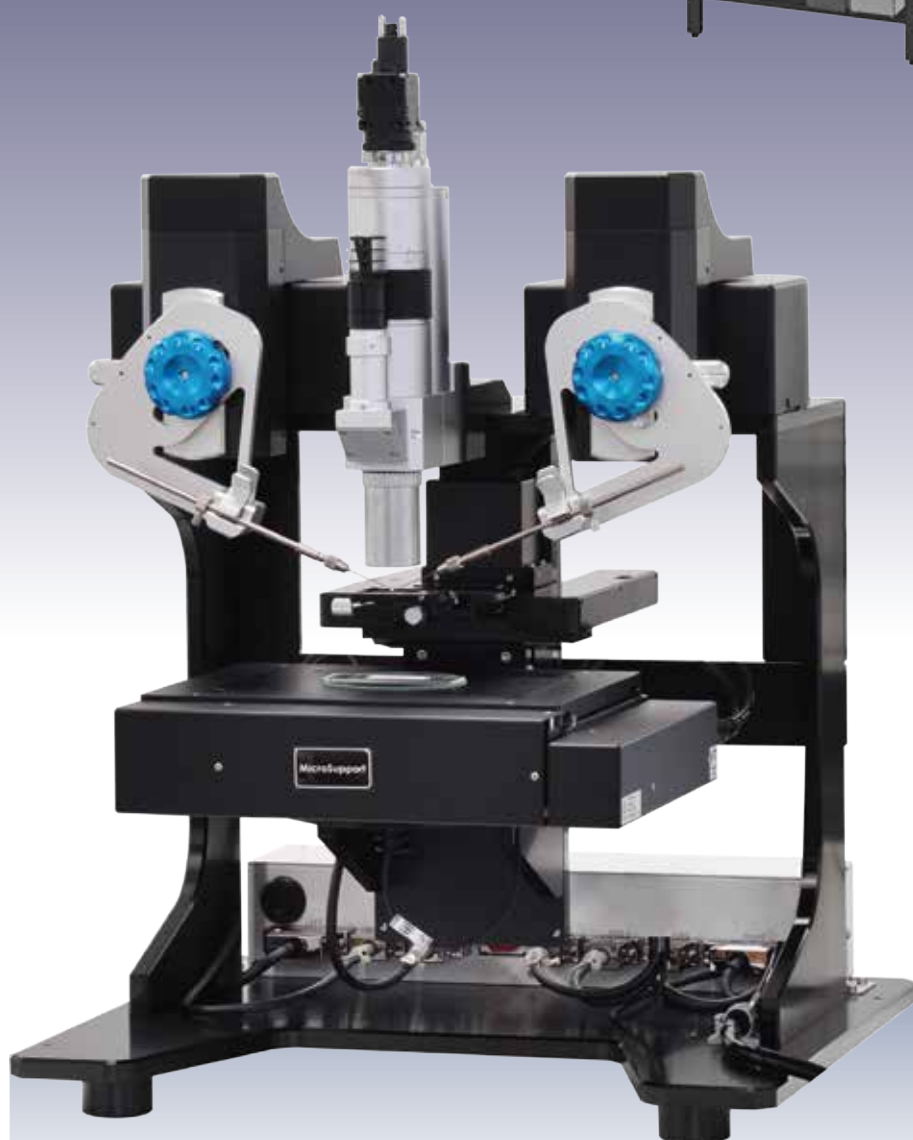
AxisPro FC without cover. Suitable for sampling inside a glovebox.
