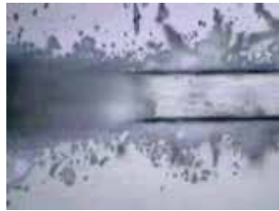
PMMA processed with flat chisel
