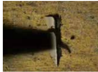
Cu processed with flat chisel
