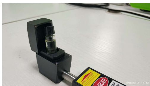
Fig 9 Sample cell for fluid (Thermo bottle)
