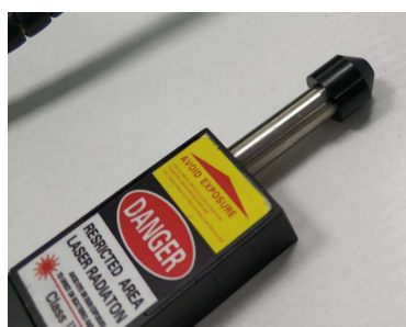
Fig 8 Raman probe for solid, power
