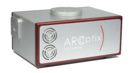
The ARCoptix FT-MIR Rocket is a highly performant, compact and reliable spectrometer that is ideal for various applications in the mid-infrared. The concentration levels of  $CO_2$  or  $H_2O$  in the interferometer volume are conveniently minimized thanks to a homemade, replaceable dessicant capsule. Thanks to its permanently aligned interferometer and solid-state reference laser, the FT-MIR Rocket offers excellent stability in both intensity and wavelength scales.
