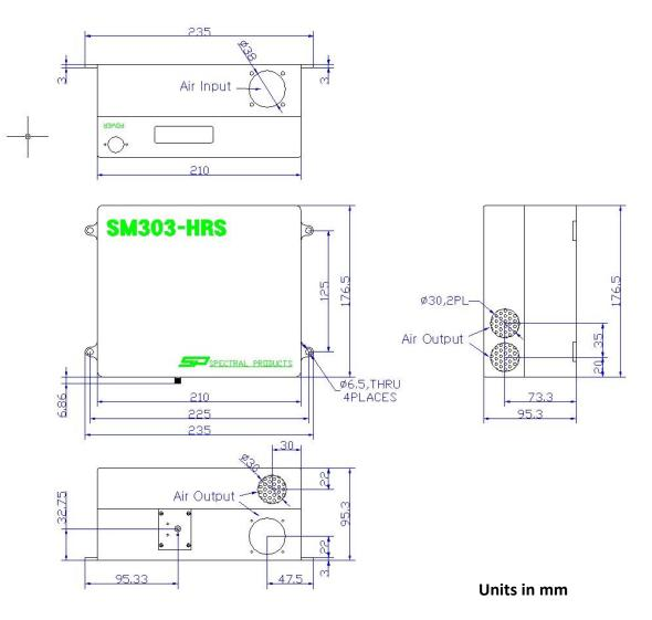
Ordering Information : Please indicate product number plus description when ordering SM303-HRS High Resolution Spectrometer w/1024-pixel CCD SM303-HRS-2048 High Resolution Spectrometer w/2048-pixel CCD
