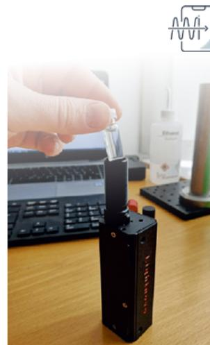
pixel quantum efficiency (QE) variation, laser optical isolation and achieving high spectral resolution. As result a novel optics miniaturization strategy allows us to create **compact Raman spectrometers and microscopes** based on non-stabilized laser diodes, densely-packed optics, and non-cooled small pixel size sensors.
