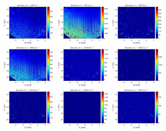
Figure 4. Spatial distributions of the spectral peak intensity at  $v = 297 \text{ cm}^{-1}$ ; 521.1 cm<sup>-1</sup>; 837.9 cm<sup>-1</sup>; 960.3 cm<sup>-1</sup>; 1278.9 cm<sup>-1</sup>; 1601.1 cm<sup>-1</sup>; 2184.3 cm<sup>-1</sup>; 2846.7 cm<sup>-1</sup>; 3247.2 cm<sup>-1</sup>.
