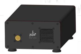
The NLIR MIR Spectrometer is based on a novel measurement scheme that upconverts the MIR light to near-visible light. Silicon-based near-visible light detectors are far superior to MIR light detectors in terms of detectivity, speed and noise. The NLIR upconversion technology therefore brings these attractive features, and the advantages that follow, to the MIR regime.
