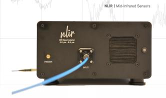
The NLIR S2050 MIR Spectrometer is based on a novel measurement scheme that upconverts the MIR light to near-visible light. Silicon-based near-visible light detectors are far superior to MIR light detectors in terms of detectivity, speed and noise. The NLIR upconversion technology therefore brings these attractive features, and the advantages that follow, to the MIR regime.
