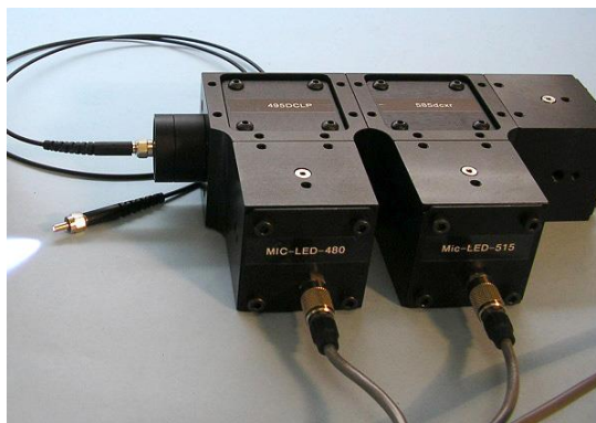
Fig. 2: Multi-wavelength light source assembled by 3 x Mic-LED, 2 x Beam Combiners, 1 x Fiber Coupled Adaptor.
