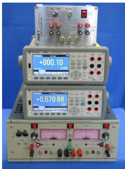
Elements of Abet 15295 Universal load, 10A capacity
