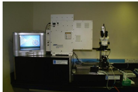
Abet Technologies Model 12002 200 W Hg source with a mask aligner for SU-8 based MEMS.
