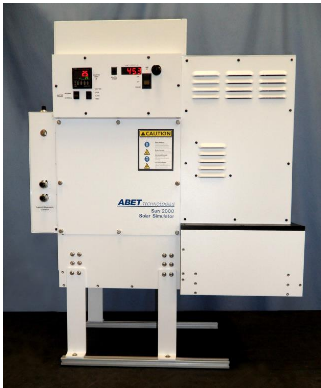
Abet Technologies Model 11044 Sun 2000 203 x 203 mm Solar Simulator.
