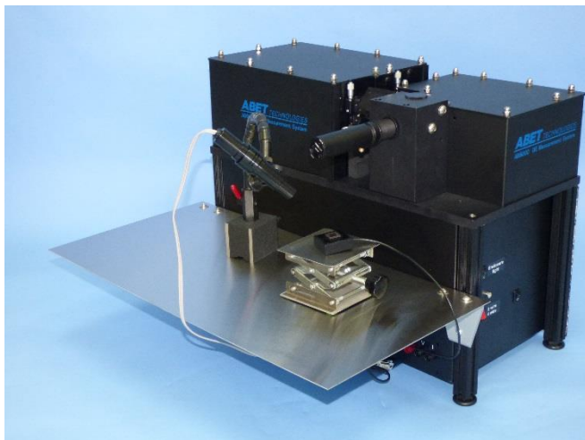
Abet Technologies Model AB6000 Quantum Efficiency measurement tool (dark enclosure not shown)
