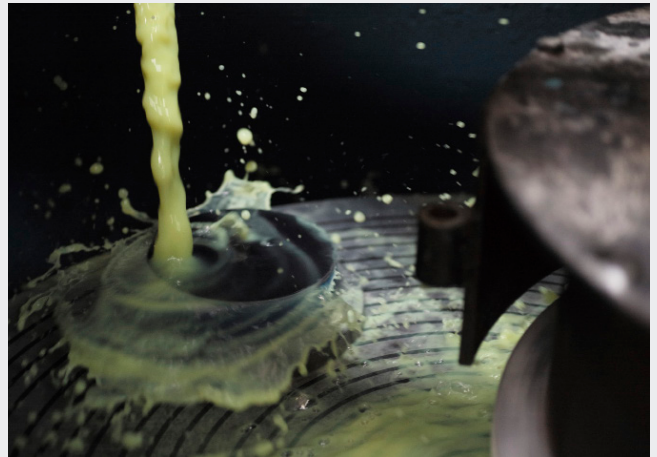
Figure 1: A Blank undergoing shaping/rough grinding
