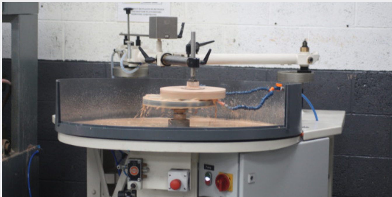
Figure 3: A pitch polisher consisting of a pitch lap and a motorised overarm for the workpiece.
