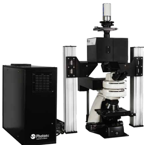
Upright configuration coupled with a CCD camera
