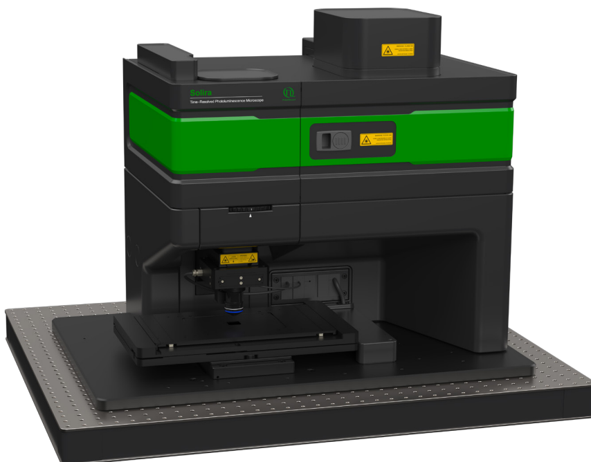
Figure 2: PicoQuant's Solira, a time-resolved photoluminescence microscope used for spatially resolved steady-state and time-resolved measurements in materials science applications.
