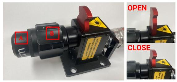
OPTICAL HEAD [A] – Focusing lens (F=30, 50, 100 or 200mm) [B] – Rotation element for focus adjustment
