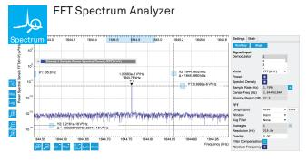
The Spectrum Analyzer takes any of the demodulators' signals or frequency as an input and applies a fast Fourier transform. The main features are:
