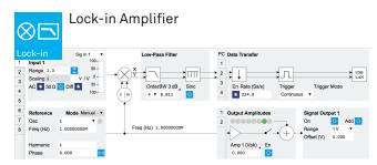
Every demodulator has a graphical representation in the form of a block-diagram for intuitive instrument. In addition, the overview tab allows the control of all demodulators, signal inputs and signal outputs from a single panel.
