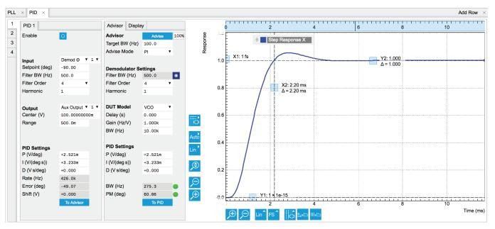
Each of the 4 PID controllers has a dedicated tab with the main controller settings in the left section, the DUT model settings and auto-tune further to the right and a large diagram to see the modelled transfer function or step-response.
