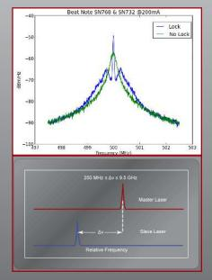
The D2-250 allows you to conveniently create a heterodyne beat note between a master and a slave laser. Typically, this beat note is delivered via a MM fiber to the D2-160 Beat Note Detector for conversion to an electrical signal. From there, the signal is processed by the D2-135 Offset Phase Lock Servo. A servo signal is produced which will create a true phase lock between master and slave with user-adjustable offset frequency of between 250 MHz and over 9.5 GHz.
