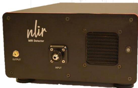
The greatest challenge for mid-infrared detectors is typically the substantial inherent noise and that they collect large amounts of radiation from the surroundings. Our detectors alleviate both limitations by using narrowband and efficient upconversion technology together with low-noise silicon-based detectors.
