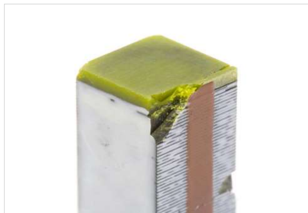
Defect of a piezostack due to non-symmetrical forces to the edge of the ceramic
