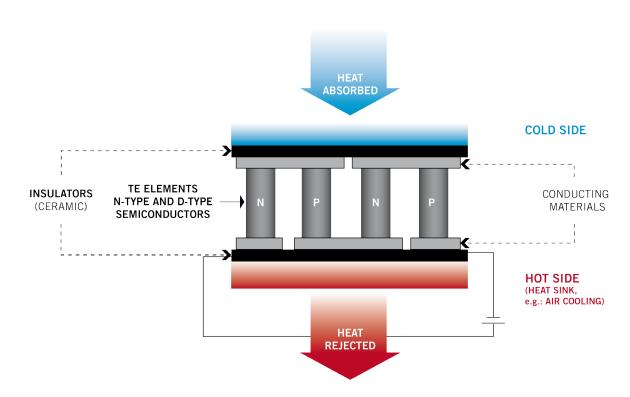
Schematic of a thermoelectric device where the Peltier effect is used to generate heat flow between two materials.
