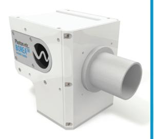
Photon etc is developing a new, affordable SWIR camera sensitive from 800 nm to  $2.6~\mu m.$  Using a stirling micro cooler, our BOREATM Camera reaches noise levels lower than its TE cooled competitors. First designed to increase the signal-to-noise ratio for faint flux applications such as hyperspectral imaging, this camera is also perfectly suited for spectroscopy, astronomy, or industrial applications.
