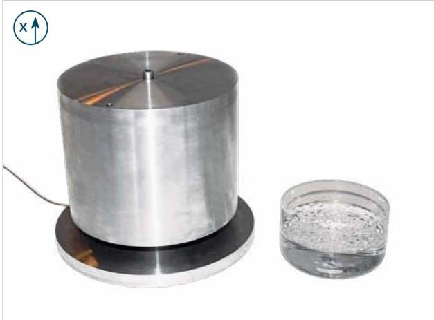
Geo-Shaker with a glass of water to show the vibration
