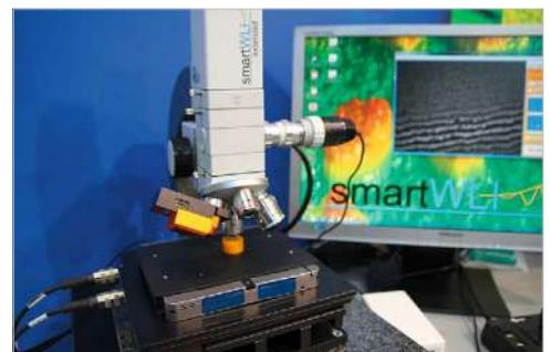
*3d surface measurement system smartWLI-microscope*
