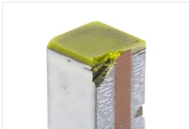
*Defect of a piezostack due to non-symmetrical forces to the edge of the ceramic*
