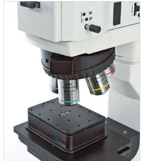
*Piezo Stack PZ Series with an accuracy below 10 nm*
