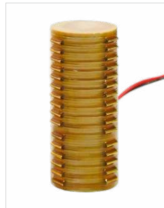
Figure 1: Piezocomposite stack actuator made from single piezoceramic discs and intermediate metal electrodes
