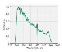
Fig 8. Typical output spectra of UltraFlux FF5010-F10 system
