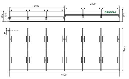
Fig 11. Typical UltraFlux FF5010-F10 laser system external dimensions
