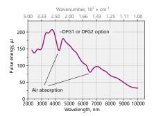
Fig 4. Typical PG501-DFG1 tuning curve
