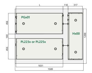
Fig 7. Recommended arrangement of pump laser and PGx01-DFGx unit on optical table
