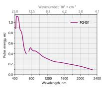
Fig 1. Typical PG401 model tuning curve Pump energy: 10 mJ at 355 nm
