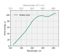
Fig 2. Typical PG401-DUV model tuning
