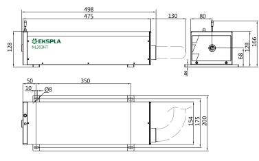
Fig 1. Typical NL300 series laser head outline drawing
