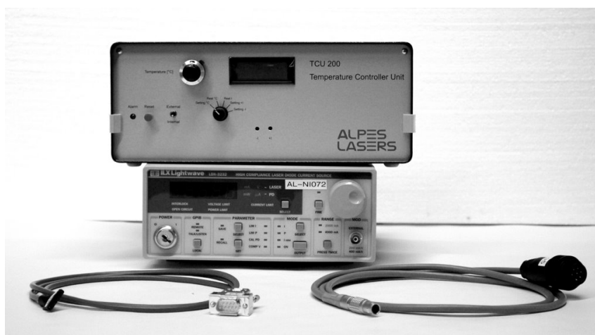
Figure 1.7.: Starter Kit for CW mode operation, shown with laser driver (not included in the Starter Kit).
