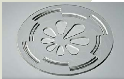
Fused-silica milling. Courtesy of FTMC.
