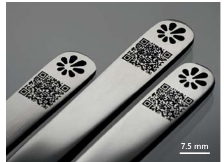
Highly-resistant black marking. Courtesy of FTMC.
