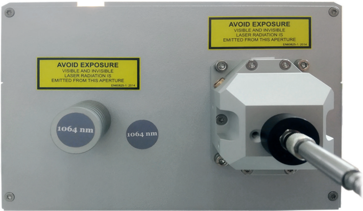
Stand-alone FCHE/NIR fiber coupler module with optional free space output
